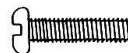
ネジ山がこまかい Narrower screw thread
